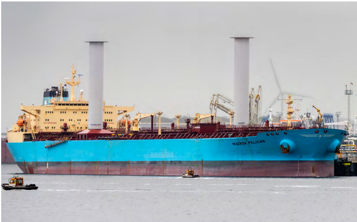
Two 30x5 Norsepower Rotor Sails on Maersk Pelican
