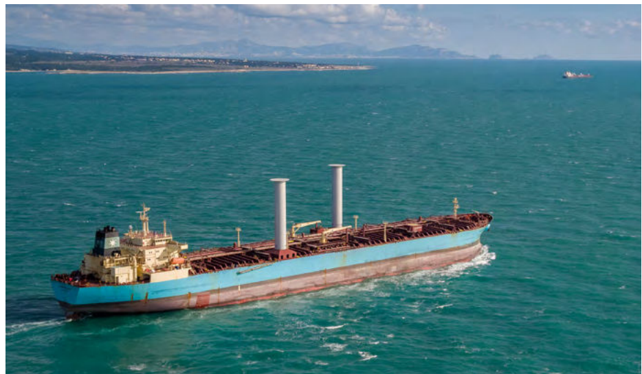
Two 30x5 Norsepower Rotor Sails on Maersk Pelican
