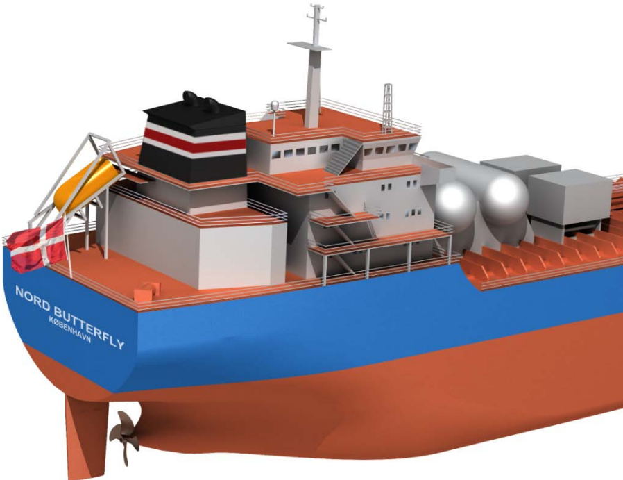
Figure 8 Aftship with LNG tanks seen from the stern
