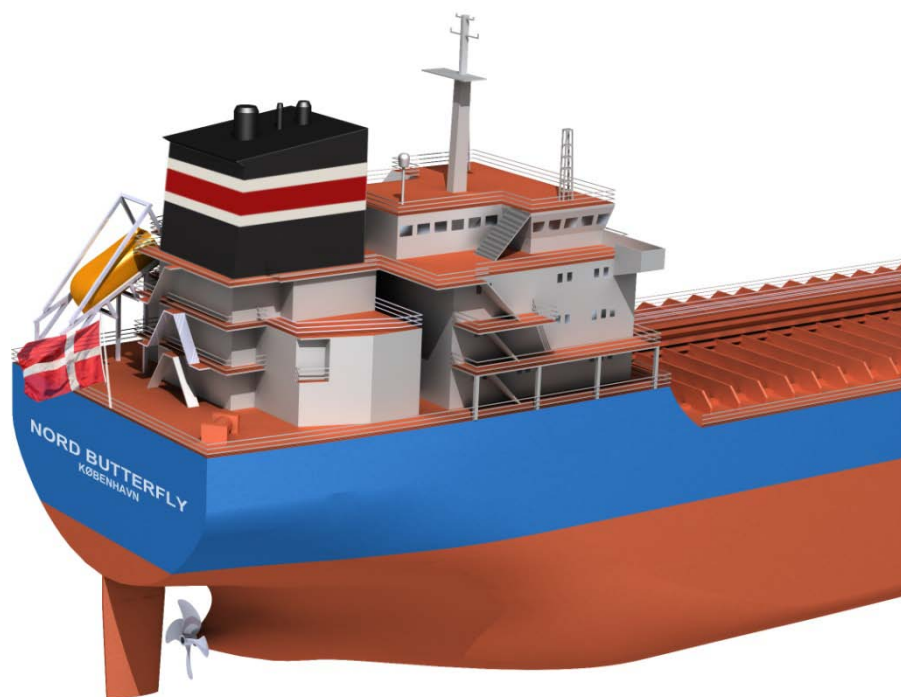
Figure 5 Aftship with scrubber installed (notice the enlarged funnel)
