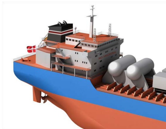
Figure 5: Aft ship with LNG tanks.
