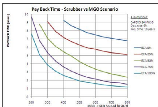
Figure 7: Payback time for scrubber for HFO at USD 650/t, global sulphur cap in 2020.
