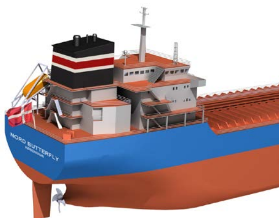
Figure 4: Aft ship with scrubber installed (notice enlarged funnel).
